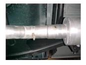
INSTALL HEAD PIPE # A ON TO YOUR EXISTING STOCK FRONT PIPE AND SECURE WITH CLAMP # F. DO NOT TIGHTEN.
