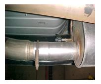
Lay out the exhaust on the floor so it looks like the drawing and compare parts with manual. To remove the stock exhaust, remove it from the clamp in front of the muffler. You may need to heat it up for easier removal. Leave all rubber grommets in place. Use WD-40 to aid in removal of exhaust and hangers.
