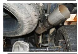
6.Be sure there is proper clearance from spare tire and shocks.
