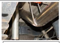
4. Install Over axlepipe Item #C onto the extension pipe. You may need to make some adjustments to find the correct location of the over axle pipe.
