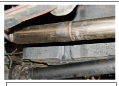
3.Install the supplied extension pipe. Use clamp Item# F to secure. Do not tighten.
