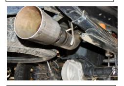
5. Install the exit pipe Item # D onto the over axle pipe. Do not tighten. Keep everything loose until you have proper clearance and exhaust tip is mounted.
