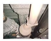
TO INSTALL YOUR GIBSON DOWN PIPE YOU NEED TO REMOVE YOUR STOCK EXHAUST FROM THE CAT BACK. REMOVE IT FROM THE 4 BOLT FLANGE IN FRONT OF YOUR STOCK MUFFLER. CUT OFF YOUR STOCK TAILPIPE FOR EASIER REMOVAL. LEAVE ALL RUBBER GROMMETS IN PLACE. USE WD-40 TO AID IN REMOVAL OF EXHAUST AND HANGER MOUNTS.
