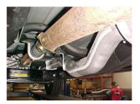
INSTALL MUFFLER # C ONTO DOWN PIPE #B 1-1/2" TO 2" USE A JACK STAND TO SUPPORT THE MUFFLER. USE CLAMP #F TO SECURE THE MUFFLER TO THE DOWN PIPE. DO NOT TIGHTEN. MUFFLER INLET IS LOOKING INTO THE LOUVERS.
