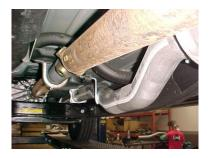
INSTALL DOWN PIPE #B ONTO DOWN PIPE #A. USING GASKET # H AND BOLT KIT # G. INSERT WELDED HANGER INTO RUBBER GROMMET. DO NOT TIGHTEN.
