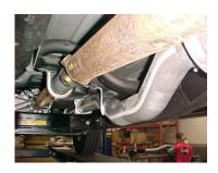
INSTALL MUFFLER # C ONTO DOWN PIPE #B 1-1/2" TO 2" USE A JACK STAND TO SUPPORT THE MUFFLER. USE CLAMP #F TO SECURE THE MUFFLER TO THE DOWN PIPE. DO NOT TIGHTEN. MUFFLER INLET IS LOOKING INTO THE LOUVERS.
