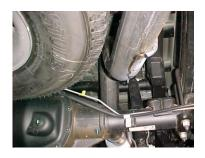
INSTALL THE OVERAXLE TAIL PIPE #D INTO THE MUFFLER 1½"-2", SECURE TO MUFFLER USING CLAMP #F. INSERT WELDED HANGERS INTO RUBBER GROMMETS. DO NOT TIGHTEN.
