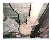
TO INSTALL YOUR GIBSON DOWN PIPE YOU NEED TO REMOVE YOUR STOCK EXHAUST FROM THE CAT BACK. REMOVE IT FROM THE 4 BOLT FLANGE IN FRONT OF YOUR STOCK MUFFLER. CUT OFF YOUR STOCK TAILPIPE FOR EASIER REMOVAL. LEAVE ALL RUBBER GROMMETS IN PLACE. USE WD-40 TO AID IN REMOVAL OF EXHAUST AND HANGER MOUNTS.
