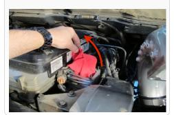
14. Reinstall your S&B or OE elbow. Be sure all connections are secure and properly positioned. Torque all hardware to the recommended specs. Reconnect the negative battery cables. The installation is now complete.
