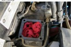
11. Place the Heater Delete (A) on top of the Bottom gasket (C), make sure all four bolt holes line up correctly.
