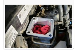
12. Place the supplied Top Gasket (B) (the one with a smaller opening) on the Heater Delete (A), make sure all four bolt holes in the gasket line up correctly.
