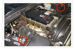
2. Loosen the upper hose clamp at the OE or S&B elbow and disconnect the hump hose from the elbow. **Note:** Care should be taken not to let any debris fall into the boost tube.
