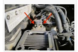
7. Follow the power cable(s) that run from the heater block to the relay(s) next to the passenger side battery. There four connection points; one under the plastic cover to the right of the heater block, two steel clips in front of the motor, and one top of the alternator bracket. Undo all connections.
