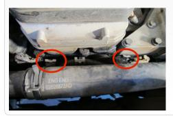
8. Disconnect the power cable(s) from the relay(s). Remove the cable(s) from the truck. Return the nut(s) to the relay(s).
