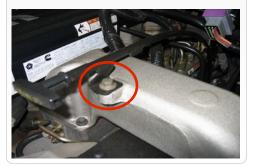
4. Remove the lock nut and pull the prong out that secures the wiring harness to the elbow and push the harness back away from the elbow. (Ignore this step if you have an S&B elbow)
