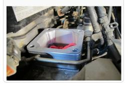
13. Remove your shop rag (if used) from the manifold and use a vacuum in the manifold to remove any debris that may have fallen in.
