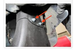
16. On the frontside of the assembly, secure the Scoop Base to the Channel using the two 1/4"-20 Screws (B), 1/4" Split Lock washers (K), and 1/4" Flat Washers (A).
