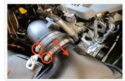
4. Remover the M8x1.25x40mm Allen Head screw from the air box and remove the complete air box assembly from the truck.
