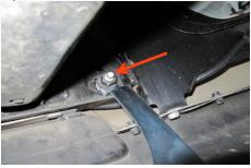
2. On the backside of the assembly, remove the two 1/4"-20x1.0" Screws (B), 1/4" Split Lock washers (K), and 1/4" Flat Washers (A) mounting Scoop base to the channel.
