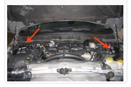
2. Disconnect the IAT sensor wiring harnesses from the sensor.
