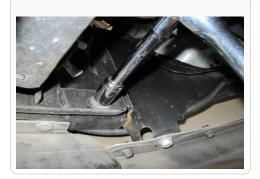
14. Slide the Scoop base assembly up into the Scoop Channel (D) and slide the mounting bracket (H) over the stud behind the bumper.
