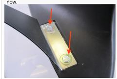
**13.** From under the truck using 18mm socket, remove the nut behind the bumper.
