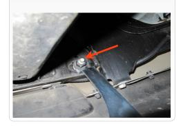
19. Check to make sure the Scoop assembly does not interfere with the wheel or wheel well liner. Turn the wheel in both directions while trying to simulate full suspension travel.
