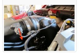
3. Loosen both the #72 Hose Clamps on the Hump adapter, then slide the hump adapter over the Filter adapter tube.
