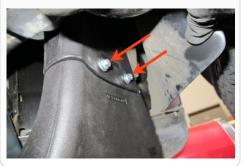
3. On the frontside of the assembly, remove the two 1/4"-20x1.0" Screws (B), 1/4" Split Lock washers (K), and 1/4" Flat Washers (A).
