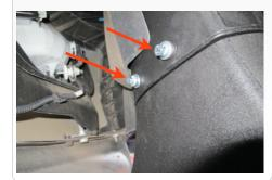
4. Install the Plug (L) into the Scoop Channel using the two 1/4"-20x3/4" Screws (M), 1/4" Split Lock washers (K), and 1/4" Flat Washers (A).
