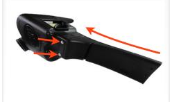
9. Slide the air box/ channel assembly down from the engine compartment and set the air box back into the two factory grommets on the side of the battery tray.
