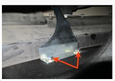
**18.** Reinstall the nut behind the front bumper securing the Mounting bracket (H). Torque to factory specs.
