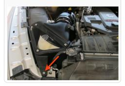
11. Install the four supplied Speed Clip Nuts (C) over the flange of the Scoop Base (E). Make sure the outside tabs snap into the holes.
