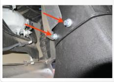
17. When you are satisfied with the positioning, tighten down the Mounting bracket (H) to the Scoop Base (E) using two 1/2" wrenches (one on top and one inside).
