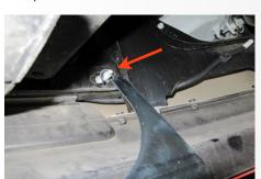
15. On the backside of the assembly, secure the Scoop Base to the Channel using the two 1/4"-20 Screws (B), 1/4" Split Lock washers (K), and 1/4" Flat Washers (A).
