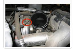
7. Loosen the V-band securing the OE inlet tube to the turbo. Then remove the OE inlet tube from the truck.
