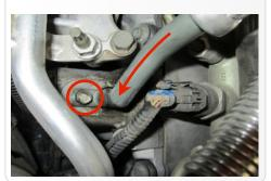
12. Use the supplied wire tie to position the small wiring harness away from the turbo and mouth piece. Clip the CCV hose back into place.
