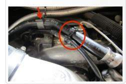
13. Re-install the S&B Intake tube (or the OE intake tube) that was removed in Step #2. Tighten all the hose clamp connections.
