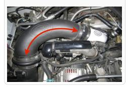
14. Tighten the V-band clamp at the turbo when you are satisfied with the positioning.
