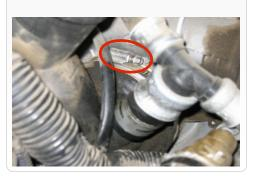
8. Install the S&B Turbo Mouthpiece (A) onto the turbo inlet using the OE V-band clamp. Be sure both flanges mate in the V-band clamp evenly. Leave the connection slightly loose for now.
