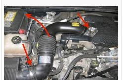
3. Remove the OE resonator by loosening the hose clamp at the turbo inlet tube and the stud towards the front using a T-30 Torx bit.
