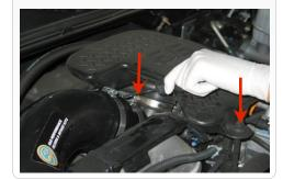
4. Using a 10mm socket, remove the screw mounting the CCV tube on the Passenger side. Pull the tube up out of the port. Save the screw for re-mounting.
