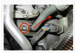
**5.** Unclip the CCV hose above the turbo. Using pliers to loosen the clamp, disconnect the CCV line from the OE inlet tube.
