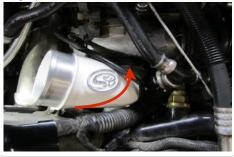
$9. \ \ \text{Using a needle nose pliers, pull the inner } \\ \text{OE hose support out of the CCV hose.}$
