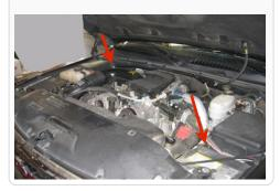
2. Loosen the clamps on either end of the S&B intake tube (or the OE Intake tube) and remove the tube from the truck.
