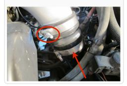
20. Secure the dip stick tube upper bracket to the Elbow. Apply thread locker to the 5/16" x 1/2" Bolt (B). Then place the Flat Washer (A) on the 5/16" x 1/2" Bolt (B). Place the bolt and washer through the upper bracket and place the Rubber Washer (M) and the other Flat Washer (A) under the bracket and thread the bolt into the elbow and secure. Do not exceed 30 In. lbs. Then tighten the two bolts at the lower bracket
