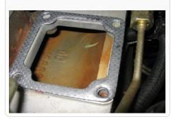
8. This kit has 2 long studs (J) and 2 short studs (H), to determine the correct stud length for your truck, thread each a long and short stud (short threaded end first) into the manifold bolt holes farthest from the valve cover. Measure the height of the stud from the heater grid block upward. Use the studs that are approximately 1.125" tall.
