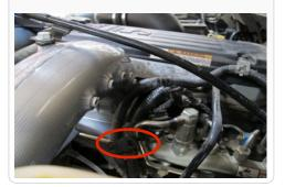
22. Reconnect both batteries. Inspect your installation, make sure the kit is properly positioned and all fasteners are secure. Affix the CARB sticker near the intake kit. The installation is now complete
