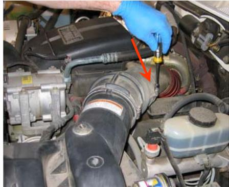
**7.** Pull up, then push the OE air box toward the engine to gain access to the air temp. sensor, disconnect the sensor.
