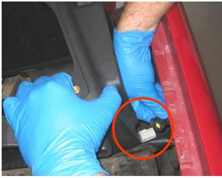
15. When the S&B air box is in place, secure using the OE nut and washer.
