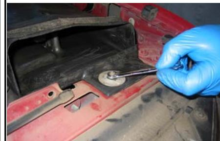
19. Install the S&B air filter (C) to the S&B air box adapter (H), secure the # 72 hose clamp.
