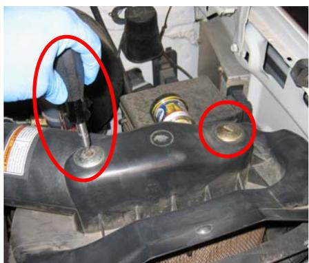
**8.** Pull up and push towards the firewall to release the OE air box from the rubber grommets, remove it and the grommets from the vehicle.
