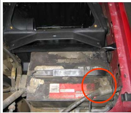
18. Reinstall the OE air scoop and secure with the OE bolt and washer.
