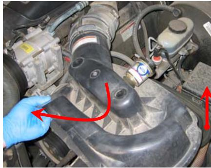
**9.** Twist a 1/4 turn to remove the OE temp. sensor from the OE air box.
