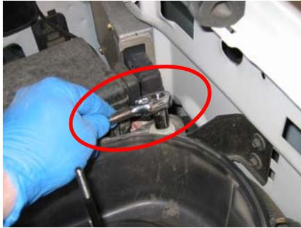
**10.** Install the OE temp. sensor onto the side of the S&B air box (F). **Type "A"** will require a Grommet (K) to be installed in the S&B air box (F) first. **Type "B"** will not, simply unscrew the sensor's 1/4 turn adapter nut and place the sensor through the hole in the box and secure using the 1/4 turn adapter nut.
