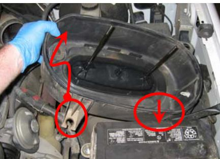
**11.** Install 2 S&B Grommets (K) into the bottom of the S&B air box (F)
