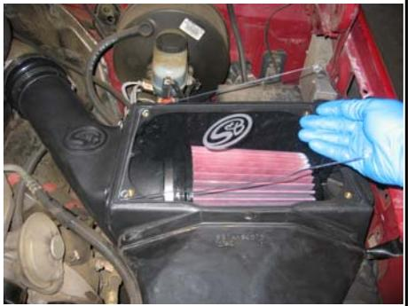
21. Inspect your installation, make sure kit is properly positioned and all fasteners and connections are tight.
