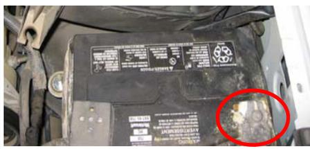
**6.** Remove the OE air box mounting nut and washer.
