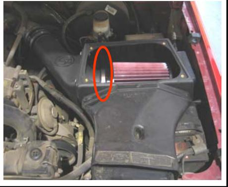
20. Install the S&B clear lid (R), secure with 10/24 screws (S) and concave rubber footed washers (U). Do not over tighten.
