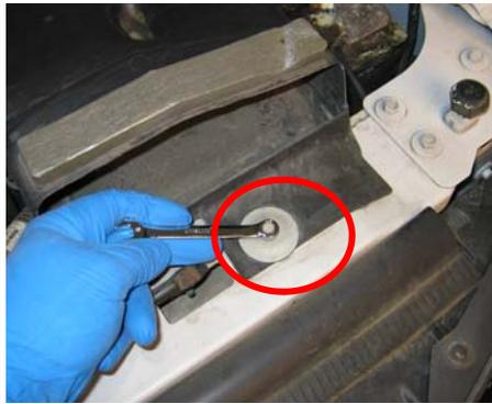
**5.** Remove the OE air box lid and tube assembly, then remove the OE air filter.
