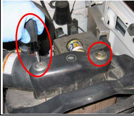
7. Pull up, then push the OE air box toward the engine to gain access to the air temp. sensor, disconnect the sensor.
