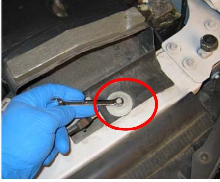
4. Remove the 2 OE air filter retaining fasteners. Use a flat head screwdriver.
