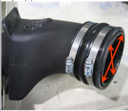
13. Attach the S&B air box adapter (H) to the S&B air box (F), latch the bottom and use the 5/16 screws (G) to secure the top.
