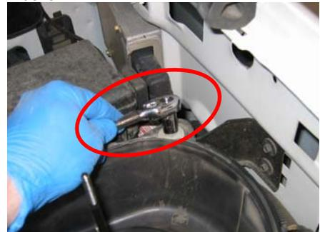
9. Twist a 1/4 turn to remove the OE temp. sensor from the OE air box.
