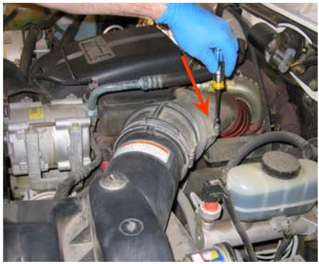
6. Remove the OE air box mounting nut and washer.
