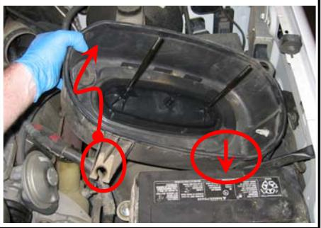
3. Loosen the OE hose clamp at the air intake tube to turbo inlet tube.
