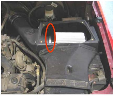
20. Install the S&B clear lid (R), secure with 10/24 screws (S) and concave rubber footed washers (U). Do not over tighten.
