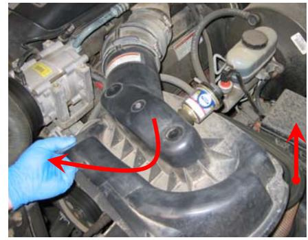
8. Pull up and push towards the firewall to release the OE air box from the rubber grommets, remove it and the grommets from the vehicle.
