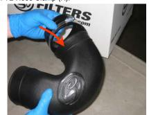
Loosen the hose clamp at the turbo inlet, then unclip the air box top and remove the OE intake tube and air filter.
