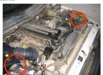
5. Determine whether your vehicle has SAE or Metric threaded studs and use the appropriate 1/4-20(F) or M6(L) lock nuts supplied and fender washers to secure the S&B air box (H) to the inner fender.
