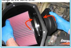
11. Install the S&B air intake tube (P) to the turbo inlet, secure the # 64 hose clamp (M).
