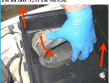
7. Attach the S&B Filter Adapter (I) to the S&B Air box (H) while slipping the air filter over the flange at the same time.
