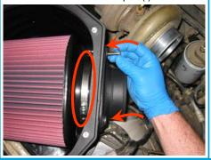
Slide the S&B Hump Adapter (Q) over the filter adapter (I), center over the gap between the tubes and secure the #72 Hose Clamps (K).
