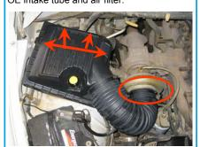
6. Place the S&B air filter (D) into the S&B air box (H).
