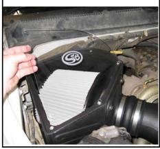
**11.** Install the S&B air intake tube (P) to the turbo inlet, secure the # 64 hose clamp (M).
