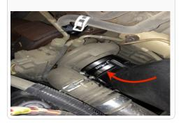
14. Slide the Hump Adapter (G) over the Intake tube (C).
