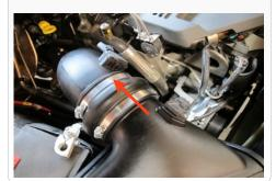
15. Make sure the Intake tube (C) and Adapter tube (I) are aligned up top and tighten the hose clamp at the turbo connection. Then tighten the #72 Clamps (F) on the Hump Adapter.
