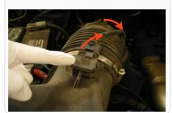
3. Loosen the hose clamp at air box lid and unsnap the clamps to remove the air box lid and stock air filter.
