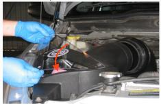
18. Reconnect both batteries. Inspect your installation, make sure the kit is properly positioned and all fasteners are secure. Affix the CARB sticker near the intake kit. The installation is now complete.
