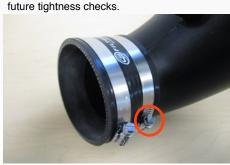
Install the S&B Air Filter (O) to the Filter Adapter (I) and secure the #80 Hose Clamp (H). Position so the flat side of the oval pointing upward parallel to the edge of the adapter
