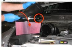
13. Install the Intake tube assembly by pushing the silicone adapter over the turbo inlet. Leave loose for now.
