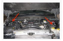
Disconnect the electrical connection for the Intake Air Temp. (IAT) Sensor, then unclip the wire loom from the tube.
