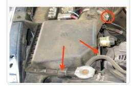
4. Remove the mounting nut then pull up and out on the lower half of the stock air box to remove it from the vehicle.
