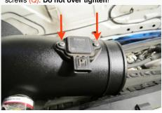
17. Push the small end of the Intake tube assembly over the turbo inlet. Leave the connection loose for now.
