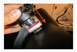
**15.** Place two #72 hose clamps (J) over the Hump Adapter (K) and slide the Hump Adapter over the Intake Tube (L) until it is flush with the end.
