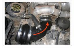
**20.** Install the Air Box (H) by placing the box at an angle so that it secures around the OE air inlet on the inner fender. Then push down until the 3 prongs slide into the OE rubber grommets. Use grease if necessary.
