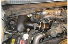
24. Remove the protective film from both sides of the Clear Lid (D), place the lid on the air box and secure using the supplied 10-24 screws (B) with sealing washers (C) and 5/16" Screws (A) with Rubber washers (S)
