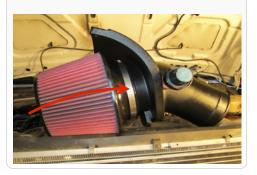
**16.** Place a #52 hose clamp (N) and a #56 hose clamp (P) on the Step Adapter (O) and secure the larger end to the intake tube.
