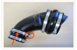
**19.** Place Air Box (H) in the area of the installation and insert the OE hot air into <u>Plug</u> for warm weather conditions or the <u>Hole</u> for cold weather conditions.
