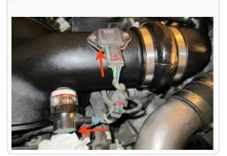
23. Use the #16 hose clamp (M) to secure the crank case breather vent line to the Intake Tube (L). It may be necessary to remove the other OE clamp and reposition the line. Then you will use the other #16 clamp and secure.
