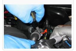
**13.** Attach the S&B Filter (E) to the Filter Adapter (G), secure with the #80 hose clamp (F).
