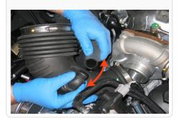
14. Remove the MAF sensor for the OE cover and attach the MAF sensor to the Filter Adapter (G). Use the MAF Gasket (I) and the OE screws. For 2009 models use the supplied M4 screws (Q). **Do not over tighten**!
