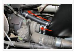
20. Make sure the Intake tube (C) and Adapter tube (K) are aligned up top and tighten the hose clamp at the turbo connection. Also tighten the hose clamp at the crankcase breather connection.
