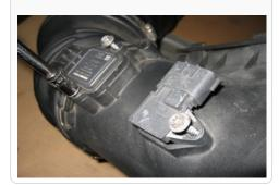
Remove the plastic clip holding the coolant overflow tube to the fender. Remove the clip from the tube and rest the tube on the air inlet foam.
