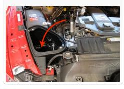
17. Attach the Air Box (Q) using the supplied M8x1.25x40mm Allen Head screw (R).
