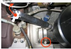
5. Remove the mounting nut on the stock air hox
