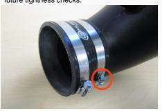
11. Slide the Breather hose over the spout on the Intake tube (C). Slide both #12 Hose clamps (X) over the hose and tighten the clamp on the spout.
