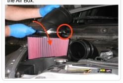
19. Install the Intake tube assembly by sliding the breather hose over the steel tube on the truck. Then push the silicone adapter over the turbo inlet. Leave loose for now.
