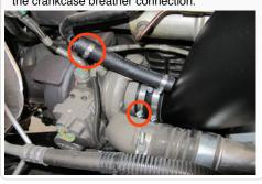
21. Slide the Hump Adapter (G) over the Intake tube (C) and secure both the #72 Hose Clamps (H).
