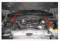
Disconnect the electrical connection for the Intake Air Temp. (IAT) Sensor and the Mass Air Flow (MAF) Sensor then unsnap the wire loom from the tube. (See the next step
