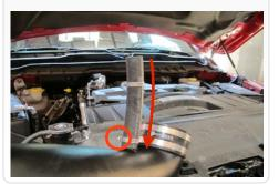
12. Place the Adapter tube (K) into the base of the S&B Air Filter (J) and tighten the #88 Hose clamp.
