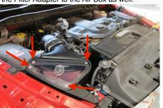
24. Reconnect both batteries. Inspect your installation, make sure the kit is properly positioned and all fasteners are secure. Affix the CARB sticker near the intake kit. The installation is now complete
