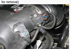
3. For the MAF sensor, Slide the red locking tab up then depress the black lever while disengaging the connector. For the IAT sensor just depress the grey lever while disengaging the connector.
