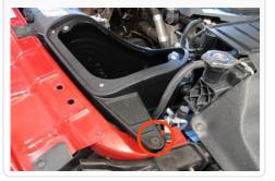
18. Carefully place the filter assembly into the Air Box trying not to ding or gouge the wire mesh. Rotate the Filter Adapter assembly into position and hook the clip into the Air Box.
