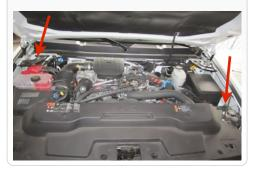
2. Disconnect the electrical connection for the Mass Air Flow (MAF) Sensor.
