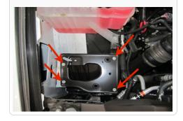
7. Between the battery and the fender; remove the nut mounting the coolant reservoir.
