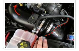
18. Slide the Hump Adapter (M) over the Intake Tube (L). When satisfied with the positioning, tighten the two #80 hose clamps (N) and #72 Hose clamp (R) at the turbo.
