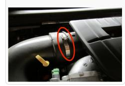
4. Loosen the hose clamp connecting the intake tube to the air box lid. Then remove the intake tube from the truck.
