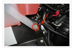
$9. \ \ \text{Remove the MAF sensor from the OE}$ air box lid. Using the two supplied #8-32 Screws (Q) and Plastic Spacers (P), install the MAF sensor into Intake Tube (L). Do not over tighten.
