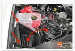
6. Remove the four bolts mounting the air box tray. Remove the mounting tray from the truck. Save all hardware.
