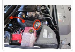
5. Remove air box lid and air filter by removing the two screws by the fender. Then carefully pull the lower portion or the air box up out of the two rubber grommets.
