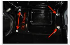
15. Reinstall the coolant reservoir mounting hardware that was removed in Steps #7 and #8.
