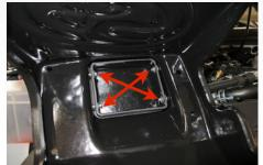
14. Move the coolant reservoir out of the way. Install the Air Box (A) using the two supplied M6x30mm screws (C) and 6mm Washers (B) for the two holes closest to the fender. Use the OE screws for the other two holes. Tighten all four.
