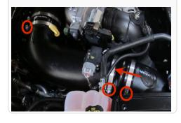
**19.** Reconnect the MAF sensor wiring harness to the MAF sensor.
