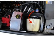
17. Route the MAF sensor wiring harness as shown. Then install the Intake Tube assembly into the Silicone adapter (R).
