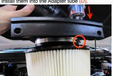
12. Slide the two #80 Hose clamps (N) over the Hump Adapter (M). Then push the Hump adapter (M) over the Adapter tube (D). Leave clamps loose for now.
