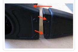
11. Secure the snorkel (Q) to the air-box (L) using the 2 Hex Head Screws (I) and washers (J).
