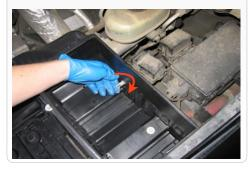
$9. \ \ \, \text{Lift the box and tray assembly up and out}$ of the vehicle. NOTE: Early 99' model OE air boxes have 2 bolts at the inner fender that need to be removed prior to the removal of the air box
