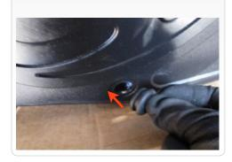
14. Install the fender seal (O) onto the air box (L).
