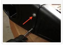
12. Use the 4 hex head screws (T) washers (N) and nuts (M) to secure the battery tray (R) to the snorkel (Q) and air-box (L).
