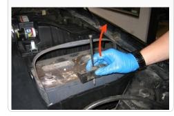
IF EQUIPPED: Disconnect the OE electronic restriction gauge electrical connector. Then, read Step #16 and plan accordingly
