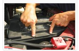
3. Remove the battery bolt and wedge then remove the battery from the vehicle.
