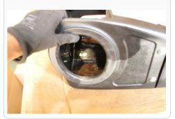
16. IF EQUIPPED: To reinstall the electronic air restriction gauge drill a 3/4" hole in the Intake Air Tube (F) at the drill point and insert the OE grommet into the hole. Then, read Step #32 to complete install.
