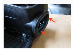
15. Install the tube seal (H) into the air box (L).
