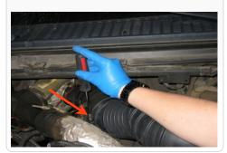
6. Unclamp and remove the OE air box lid and intake tube assembly from vehicle.
