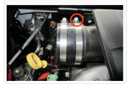
12. Place the Adapter Tube (D) into the base of the S&B Air Filter (E) and tighten the #96 Hose clamp (F). Remove the Filter minder and grommet from the OE air box lid, then reinstall them into the Adapter tube (D).
