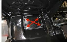
**16.** Reinstall the coolant reservoir mounting hardware that was removed in Steps #7 and #8.
