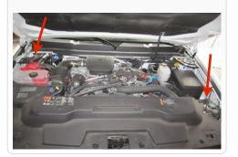
4. Loosen the hose clamp connecting the intake tube to the air box lid. Then remove the intake tube from the truck.
