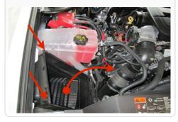
8. Unsnap the plastic clip holding the coolant reservoir to the AC line using a flat blade screwdriver. Then remove the other screw mounting coolant reservoir.
