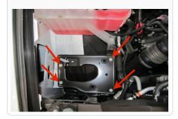
9. Remove the MAF sensor from the OE air box lid. Using the two supplied #8-32 Screws (Q) and Plastic Spacers (P), install the MAF sensor into Intake Tube (L). Do not over tighten.
