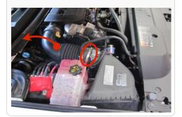
7. Between the battery and the fender; remove the nut mounting the coolant reservoir.
