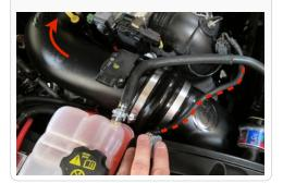
**11.** Place the Silicone Adapter (R) and both #72 Hose Clamps (O) onto the turbo inlet mouthpiece. Tighten the clamp on the turbo mouthpiece only.
