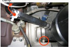
5. Loosen the hose clamp on the intake tube to assist with the removal of the air box.
