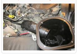
**35.** Before installing the air box and tube assembly attach the diverter harness connector to the diverter motor (L) that is located underneath the S&B air box.
