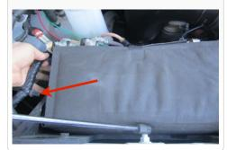
**13.** Once the push pins are pulled out the harness can be pulled out further.
