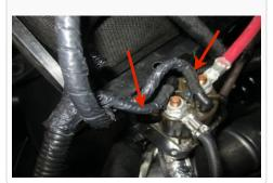
15. Disconnect the wires from the relay component by pulling them off. Please take note on which wire was connected to which terminal because these wires will be reconnected after modification. Please mark each wire or take a photo to help remember the wire connections.
