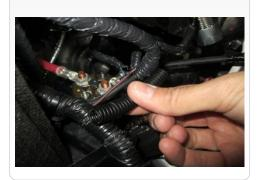
20. Install the insulated sleeve (AC) over both wires, this extra length will let the harness extend and reach the S&B air box. Re-apply electrical tape to any exposed wires and sleeve to avoid corrosion.
