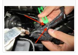
17. Once the insulation is cut at the base of each line carefully cut into the main harness and again be careful not to cut or damage the wires inside.
