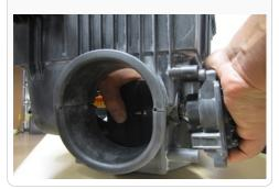
27. Mount the diverter motor onto the bottom of the S&B intake air box (I) using spacers (K) and screws (M) and washers (BB).
