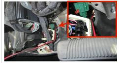
**L.** Once done running the wire through the guard, run wire down along the side of the battery. It is recommended to run the wire through the swing gate motor harness.
