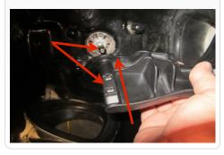
30. Note: Do NOT remove Swing Gate Arm (S) after installing it to the motor as this could damage the snap in feature of the arm. If removal of Dam (N) is desired, remove with Arm (S) installed on motor (L).
