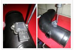
**25.** Remove the diverter intake motor (L) from the side of the factory air box using a T-27 torx key.
