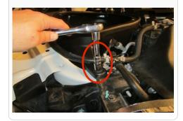
**39.** Connect hose (T) and tighten hose clamp (Y).
