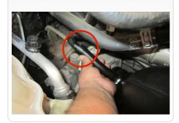
40. Connect coupler (Z) to turbo and tighten hose clamp (AA). Please make sure the coupler is push all the way onto turbo before tightening completely.
