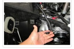
11. First remove the harness push pins that hold the harness down to the battery tray using a pry tool or flat head screw driver.
