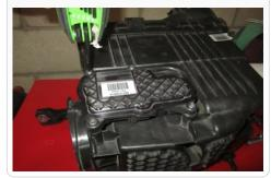
26. A good amount of force may be required to remove the motor from the factory air box. The motor shaft may need to be rotated while removing from the factory butterfly valve in the factory air box. Grab both the butterfly valve and motor and twist while pulling out.
