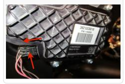
9. Once the swing gate motor is disconnected completely remove the factory air box and intake tube by lifting up and out.
