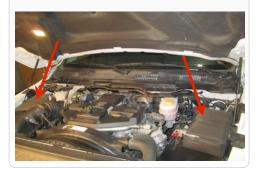
2. Disconnect the electrical connection for the Intake Air Temp. (IAT) Sensor and the Mass Air Flow (MAF) Sensor then unsnap the wire loom from the tube. (See the next step for removal)
