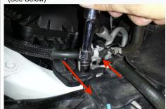
7. Lift up on factory air box, be careful not to remove the whole box because the swing gate motor harness is still connected on the side of the air box. Remember to move the hose forward from Step 6 when pulling out the box.
