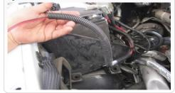
**M.** Photo of finished harness with the correct wire taps. It is recommended to use zip ties on lose wires and to also use electrical tape over the tap connectors for added protection.
