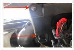
**36.(b)** Reach under the air box to feel if the posts pushed through the holes (grommets). Be careful not to push to hard or the tabs will break off the battery tray.
