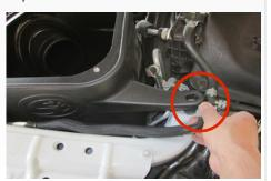
**38.** Push down on air box and tighten the provided retaining bolt (H).
