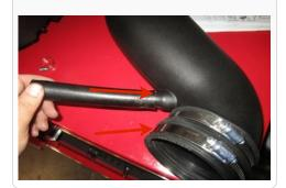
33. Install S&B intake tube (X) into S&B air box (I) by sliding the tube through the tube seal (Q). This should be a snug fit. A perfect seal is not required.
