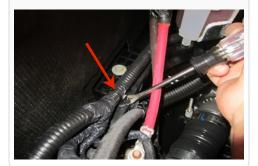
12. Remove the push pins on the harness that are located on the side and back of the battery tray.
