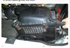
8. Disconnect the factory swing gate motor connector that is located on the side of the factory air box. Press in the locking button on the connector and pull out.
