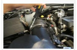
6. Remove factory retaining bolt on the front of the factory air box. Once retaining bolt is removed disconnect hose clip by pulling up and then move hose forward to help remove air box. (See Below)
