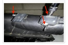
24. Place MAF sensor and IAT Sensor onto the S&B intake tube (X) using the 8-32 pan head screws (U) and gaskets (V&W).
