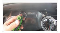
**E.** Install monitoring light (AD) into the drilled out hole, screw the locking nut onto the back of the panel by running the wire through the nut.
