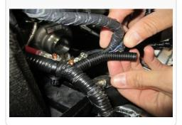
21. Once both lines are insulated with the provided insulation sleeve reconnect each wire to the correct terminal on the relay component.
