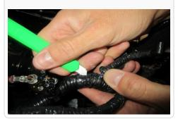
18. Once the insulation is cut pull a length of about 3 inches for each line.
