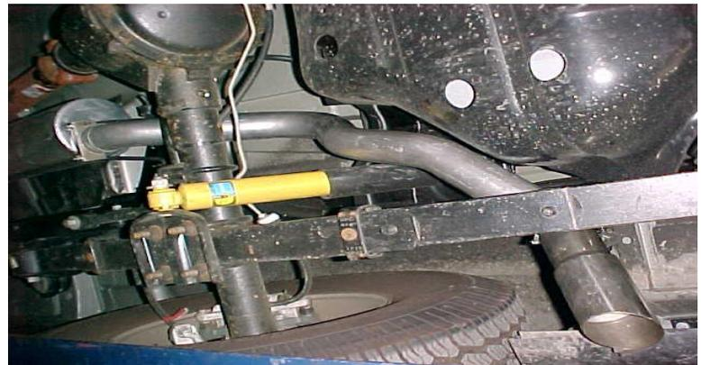
**4.** INSTALL TAILPIPE #B AND INSERT WELDED HANGER INTO RUBBER GROMMETS AND THEN INSERT IT INTO THE REAR OF THE MUFFLER. AND ATTACH WITH HANGER #D. INSTALL THE STAINLESS TIP. TO CLEAN USE ANY STAINLESS OR ALUMINUM CLEANER..
