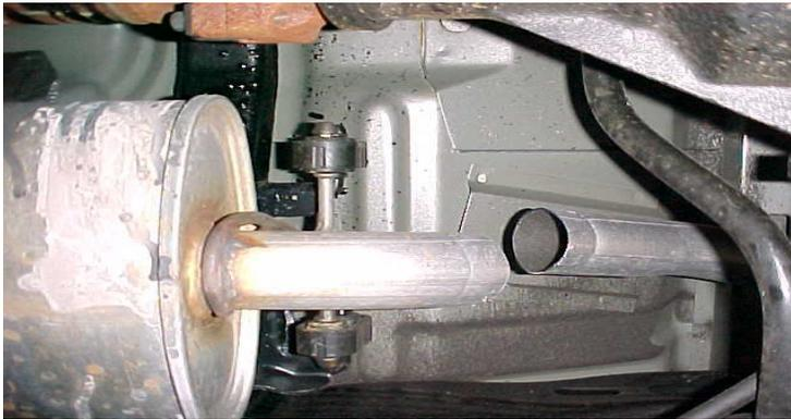
**1.** NOW, CUT STOCK TAILPIPE JUST ABOVE THE FIRST BEND COMING OUT OF THE REAR OF THE STOCK MUFFLER. REMOVE STOCK TAILPIPE .
