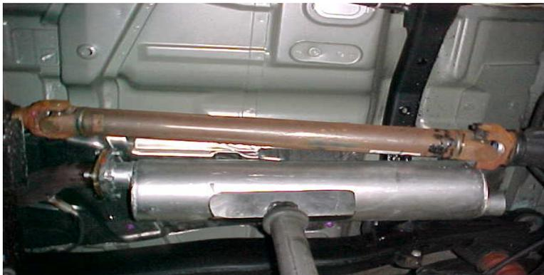
**3.** INSTALL THE MUFFLER # A TO THE STOCK FLANGE USING BOLT KIT # F AND GASKET # E WE SUGGEST USING A HIGH TEMP GASKET SEALER ON THE STOCK GASKET WHEN REINSTALLING. USE JACKSTANDS TO SUPPORT THE MUFFLER. INSTALL HANGER #D IN REAR RUBBER GROMMETS NEAR THE OUTLET OF THE MUFFLER.
