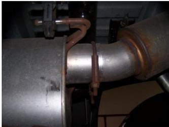
2. Remove your stock tail pipe from stock muffler by removing the clamp located on the outlet of muffler. Do not cut or damage your factory tail pipe you will re-use it. Leave all rubber grommets on the factory hangers on the vehicle.
