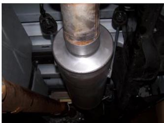
4. Install head pipe #A onto factory pipe. Use clamp #D to secure pipes together. Insert welded hangers into rubber grommets. Do not tighten.
