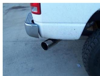
8. Install stainless steel tip. Clamp down. When you have everything in place, firmly tighten all bolts and clamps down securely. Use stainless steel cleaner and a Scotch Brite pad weekly to prevent tip from discoloration. Inspect all fasteners after 25-50 miles of operation and re-tighten as necessary. You may need to cut your stock tail pipe back to get your tip to fit correctly.
