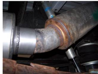
7. Re-install your factory tail pipe. Use clamp #D to secure pipe to muffler. Do not tighten. Insert hanger into rubber grommet.
