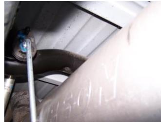
6. Install band clamp #C onto muffler. Inset hangers into rubber grommets. Use bolt kit #E to secure band clamp to muffler. Do not tighten.
