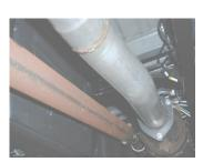
3. Install headpipe #A onto your existing stock front pipe Re-using the factory nuts.
