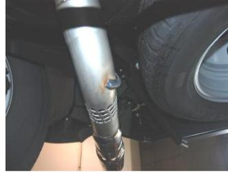
5. Adjust to fit properly then tighten all clamps and bolts. Use stainless steel cleaner to prevent tip from discoloration, Inspect all fasteners after 25-50 miles & retighten as necessary
