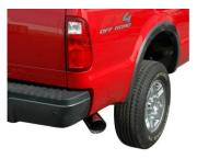
7. Install stainless steel tip. Make sure not to cover the louvers with the tip. The tip should come right up to the louvers, but do not cover. Clamp down. When you have everything in place, firmly tighten all bolts and clamps down securely. Use stainless steel cleaner and a Scotch Brite pad weekly to prevent tip from discoloration. Inspect all fasteners after 25-50 miles of operation and re-tighten as necessary. You may need to cut your stock tail pipe back to get your tip to fit correctly.
