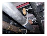
3. Install headpipe #A onto your existing stock front pipe and attach with clamp #F. Insert welded hanger into rubber grommet.
