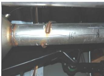
2. Short Beds: To remove your stock exhaust, Measure 16" from the end of the factory converter and Particular filter then cut. Do not damage your factory gourmets. You will re-use. them
