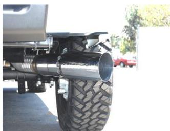
4. Next, slide exit pipe #B onto tailpipe. Use clamp #C to secure the exit pipe to the tailpipe. Do not tighten. Insert welded hangers into Rubber grommets
