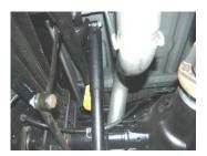
4. Install the over axle tailpipe #B onto headpipe 1.5"-2". Use clamp #D to secure. Do not Tighten
