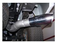
7. Next, slide exit pipe #D onto tailpipe. Use clamp #F to secure the exit pipe to the tailpipe. Do not tighten.
