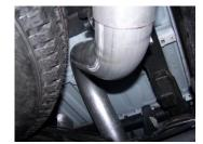
5. Slide the over axle tailpipe #C into the muffler 1.5-2". Use clamp #F to secure tailpipe to muffler. Do not tighten. Insert welded hanger into rubber grommet.
