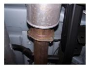
2. To remove your stock exhaust, unbolt it at the 3-bolt flange located in front of your stock muffler. Disengage the welded hangers from the rubber grommets. Use WD-40 to aid in this process. Do not damage or remove the rubber grommets as you will reuse them to mount the new system. Now, cut off the tailpipe and remove the exhaust.
