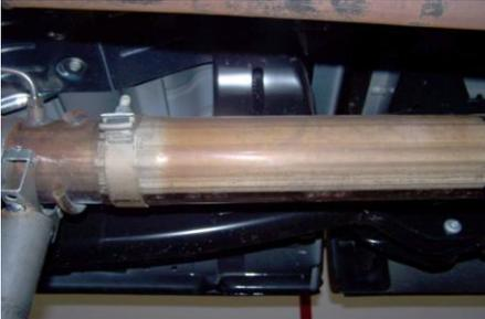
2. Install Item # A on to your factory exhaust using clamp # D to secure. Do not tighten.
