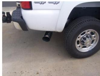
Install stainless steel tip. Clamp down. When you have everything in place, firmly tighten all bolts and clamps down securely. To clean stainless steel tips, use stainless steel cleaner and a Scotch Brite pad.
