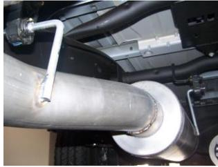
Install the over axle tailpipe #C into the muffler 1 1/2-2". Secure to muffler using clamp #E. Insert welded hanger into rubber grommet. DO NOT TIGHTEN.
