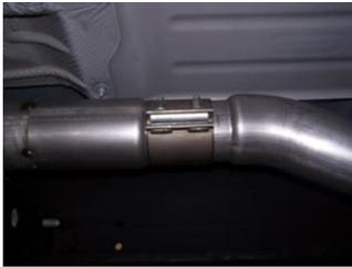
Install head pipe #A onto your factory down pipe using factory clamp to secure. DO NOT TIGHTEN. Insert welded hanger into rubber grommet.
