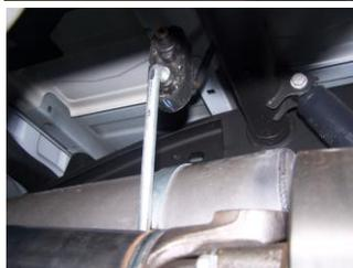
Install band clamp #D onto muffler. Use bolt kit #G to secure band clamp to muffler. DO NOT TIGHTEN. Insert welded hanger into rubber grommet.
