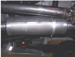
Install muffler #B onto head pipe 1 1/2-2", with louvers facing forward. Use a jack stand to support the muffler. Use clamp #E to secure the muffler to the head pipe. Muffler inlet is looking into the louvers.
