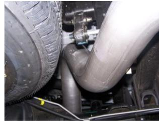
Install stainless steel tip. Clamp down.
