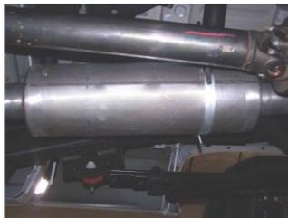
Install muffler #B onto head pipe 1 1/2-2", with louvers facing forward. Use a jack stand to support the muffler. Use clamp #E to secure the muffler to the head pipe. Muffler inlet is looking into the louvers. Install band clamp #D onto muffler. Use bolt kit #G to secure band clamp to muffler. DO NOT TIGHTEN. Insert hanger into rubber grommet.
