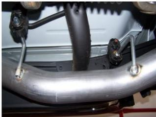
Install head pipe #A onto your factory down pipe using factory clamp to secure. DO NOT TIGHTEN. Insert hangers into rubber grommets.
