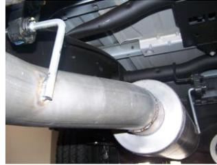
Install the over axle tailpipe #C into the muffler 1 1/2-2".
