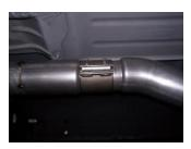
Install head pipe #A onto your factory down pipe using factory clamp to secure. DO NOT TIGHTEN. Insert welded hangers into rubber grommets.
