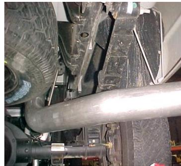
Install the turnout pipe # D on to the tailpipe. Insert welded hanger into rubber grommet. Secure together with clamp # F. Do not tighten. Roll the exit pipe until it is at the correct angle for your truck.
