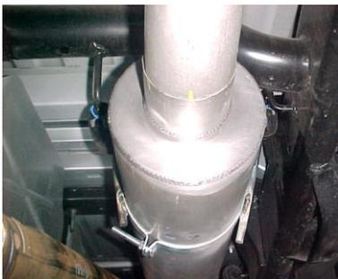
Install muffler # B onto headpipe # A 1-1/2"-2". Use clamp # F to secure to headpipe, do not tighten. Next, install band clamp # H onto muffler and insert hangers, do not tighten.
