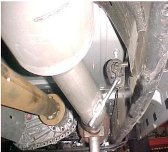
Install headpipe # A on to your existing stock front pipe and secure with clamp # G. Make sure to line up the notch. Insert welded hanger into rubber grommet. Do not tighten.
