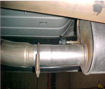
Lay out the exhaust on the floor so it looks like the drawing and compare parts with manual. To remove it from the clamp in front of the muffler. You may need to heat it up for easier removal. Leave all rubber grommets in place. Use WD-40 to aid in removal of exhaust and hangers.
