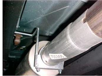
Install muffler onto head pipe # A 1-1/2" to 2" with the louvers facing towards the converter. Use a jack stand to support the muffler. Use clamp #F to secure the muffler to the head pipe. Do not tighten. Insert hanger into rubber grommet. Muffler inlet is looking into the louvers.
