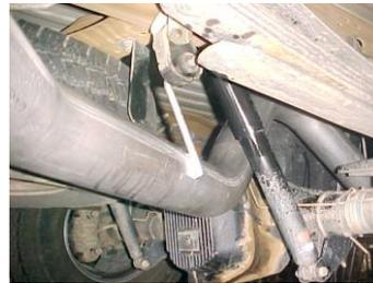
Install stainless steel tip. Clamp down. When you have everything in place, firmly tighten all bolts and clamp down securely. To clean stainless steel tip use any stainless steel cleaner and Scotch Brite pad.
