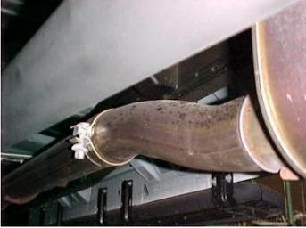
Lay out the exhaust on the floor so it looks like the drawing and compare parts with manual. To remove the stock exhaust remove it from the clamp located just in front of the muffler.
