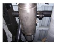
4. Slide muffler #B onto headpipe 1.5-2". Insert welded hangers into rubber grommets. Use clamp #F to secure muffler to the headpipe. Do not tighten.
