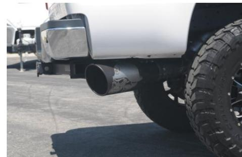
7. With proper clearance from spare tire and the tip in your desired position begin to tighten down all clamp connections from the front head pipe back to the tip.
