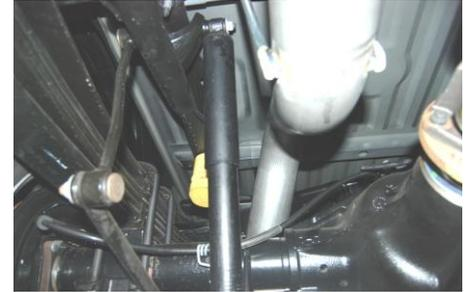
4. Install Over axle pipe Item # B onto the head pipe. Use clamp Item E to secure but do not tighten.
