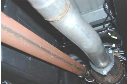
3. Install Head pipe Item #A onto the factory flange. Do not tighten until install is complete.
