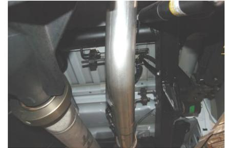
4. Install Over axle pipe Item # A onto the factory head pipe. Use clamp Item D to secure but do not tighten.
