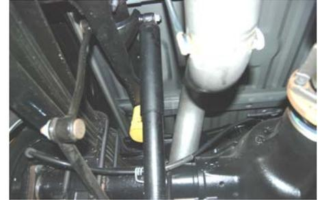
4. Install Over axle pipe Item # B onto the head pipe. Use clamp Item E to secure but do not tighten.
