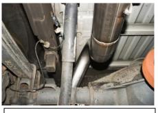
4. With the hanger placed in the rubber grommet install the over axle pipe item # B. Do not tighten.
