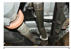
3. Install head pipe item # A onto the factory flange using factory gasket and supplied bolt. Kit. Do not tighten the flange. Keep the flange loose until the system is completely installed.
