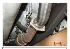
**2.** Remove the factory head pipe by un-bolting the 3-bolt flange located behind the factory DPF. Do not damage the factory gasket you will need to re use it..
