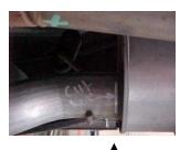
TO REMOVE STOCK EXHAUST CUT OFF YOUR STOCK SYSTEM JUST IN FRONT OF THE MUFFLER AFTER THE WELD, LEAVE ALL RUBBER GROMMETS ON THE HANGERS. USE WD-40 TO AID IN THE REMOVAL OF EXHAUST AND HANGERS.
