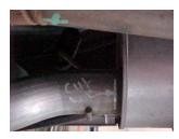
TO REMOVE STOCK EXHAUST CUT OFF YOUR STOCK SYSTEM JUST IN FRONT OF THE MUFFLER AFTER THE WELD, LEAVE ALL RUBBER GROMMETS ON THE HANGERS. USE WD-40 TO AID IN THE REMOVAL OF ECHAUST AND HANGERS.
