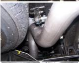
Install the over axle tailpipe #C into the muffler 1½-2". Secure to muffler using clamp #E. Insert welded hanger into rubber grommet. DO NOT TIGHTEN.
