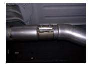
Install head pipe #A onto your factory down pipe using factory clamp to secure. DO NOT TIGHTEN. Insert welded hanger into rubber grommet.
