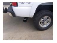
GIBSON EXHAUST systems are designed on a factory stock vehicle. Any aftermarket products installed could increase the sound levels of this Exhaust. Make sure there is a 1" clearance from ALL rubber brake lines, shock boots, fuel lines, tires, etc to prevent heat related damage or fire.
