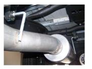
Install the over axle tailpipe #C into the muffler  $1\frac{1}{2}-2^{"}$ .
