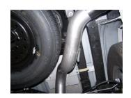
Install stainless steel tip. Clamp down.
