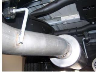
Install the over axle tailpipe #C into the muffler 1 1/2-2". Secure to muffler using clamp #D. Insert welded hangers into rubber grommets. DO NOT TIGHTEN.
