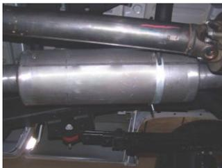
Install muffler #B onto head pipe 1 1/2-2", with louvers facing forward. Use a jack stand to support the muffler. Use clamp #D to secure the muffler to the head pipe. Muffler inlet is looking into the louvers. DO NOT TIGHTEN.
