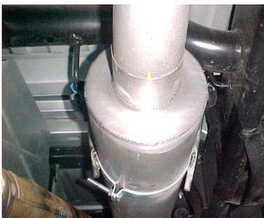
Install muffler # B onto headpipe # A 1-1/2"-2". Use clamp # F to secure to headpipe, do not tighten. Next, install band clamp # G onto muffler and insert hangers, do not tighten.
