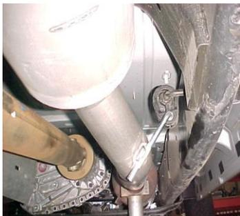
Install headpipe # A on to your existing stock front pipe and secure with clamp # F. Make sure to line up the notch. Insert welded hanger into rubber grommet. Do not tighten.
