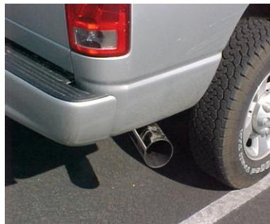
Install stainless steel tip. Clamp down. When you have everything in place, firmly tighten all bolts and clamp down securely. To clean stainless steel tip use any stainless steel cleaner.
