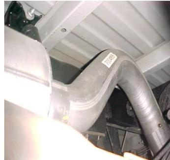
Install the over axle tailpipe # C into the muffler 1-1/2" to 2". Secure to the muffler using clamp # F. Do not tighten.
