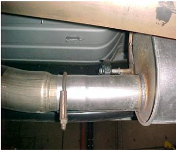
Lay out the exhaust on the floor so it looks like the drawing and compare parts with manual. To remove the stock exhaust, remove it from the clamp in front of the muffler. You may need to heat it up for easier removal. Leave all rubber grommets in place. Use WD-40 to aid in removal of exhaust and hangers.
