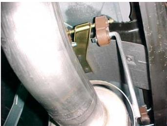
Install band clamp # G into rubber grommets located just above the axle. Do not tighten. Attach with bolt kit #J.
