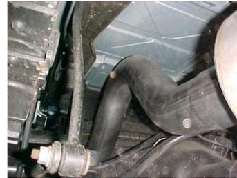
Install the over axle tailpipe # C into the muffler 1-1/2" to 2". Secure to the muffler using clamp # H Do not tighten. You may need to loosen spare tire & push over towards driverside & re tighten. Next install exit pipe # D onto overaxle pipe insert hanger into rubber grommet. Use clamp # H to secure pipes together rotate to proper angle for your vehicle. DO NOT TIGHTEN.
