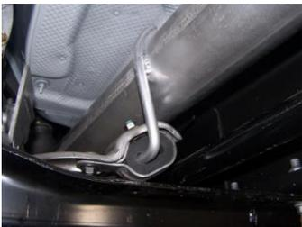
Install down pipe #A onto turbo and secure with factory clamp. **DO NOT TIGHTEN.** Insert welded hanger into bottom hole of rubber grommet.
