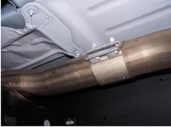
Lay out the exhaust on the floor so it looks like the drawing and compare parts with manual. To remove the stock exhaust unclamp it just in front of muffler. Save factory clamp. Leave all rubber grommets in place. Use WD-40 to aid in removal of exhaust and hangers.
