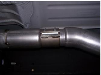
Install head pipe #B onto down pipe using factory clamp to secure. **DO NOT TIGHTEN.** Insert hanger into rubber grommet.
