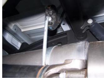
Install muffler #C onto head pipe 1 1/2-2", with louvers facing forward. Use a jack stand to support the muffler. Use clamp #F to secure the muffler to the head pipe. Muffler inlet is looking into the louvers. Install band clamp #E to support muffler, insert hanger into rubber grommet. Use bolt kit #H to secure band clamp to muffler. **DO NOT TIGHTEN.**
