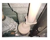
TO INSTALL YOUR GIBSON DOWN PIPE YOU NEED TO REMOVE YOUR STOCK EXHAUST. REMOVE IT FROM THE 4 BOLT FLANGE IN FRONT OF YOUR STOCK MUFFLER, CUT OFF YOUR STOCK TAILPIPE FOR EASIER REMOVAL. LEAVE ALL RUBBER GROMMETS IN PLACE. USE WD-40 TO AID IN REMOVAL OF EXHAUST AND HANGER. AFTER YOUR STOCK EXHAUST IS REMOVED YOU NEED TO REMOVE THE CATALYTIC CONVERTER.
