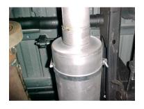
INSTALL BAND CLAMP #H ONTO MUFFLER. INSERT WELDED HANGER INTO RUBBER GROMMET. TIGHTEN BAND CLAMP USING HARDWARE KIT #I.
