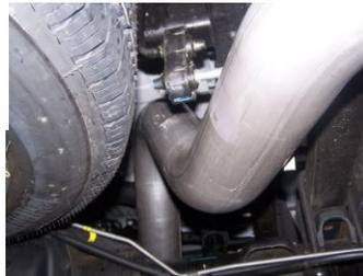
Install the overaxle tail pipe #D into the muffler 1 1/2-2". Secure to muffler using clamp #F. DO NOT TIGHTEN.
