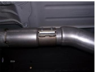
Install headpipe #B onto downpipe using factory clamp to secure. Insert welded hangers into rubber grommet. DO NOT TIGHTEN.
