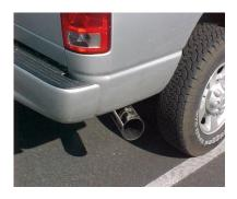
Install stainless steel tip. Clamp down. When you have everything in place, firmly tighten all bolts and clamp down securely. To clean stainless steel tip use any stainless steel cleaner and Scotch Brite pad.
